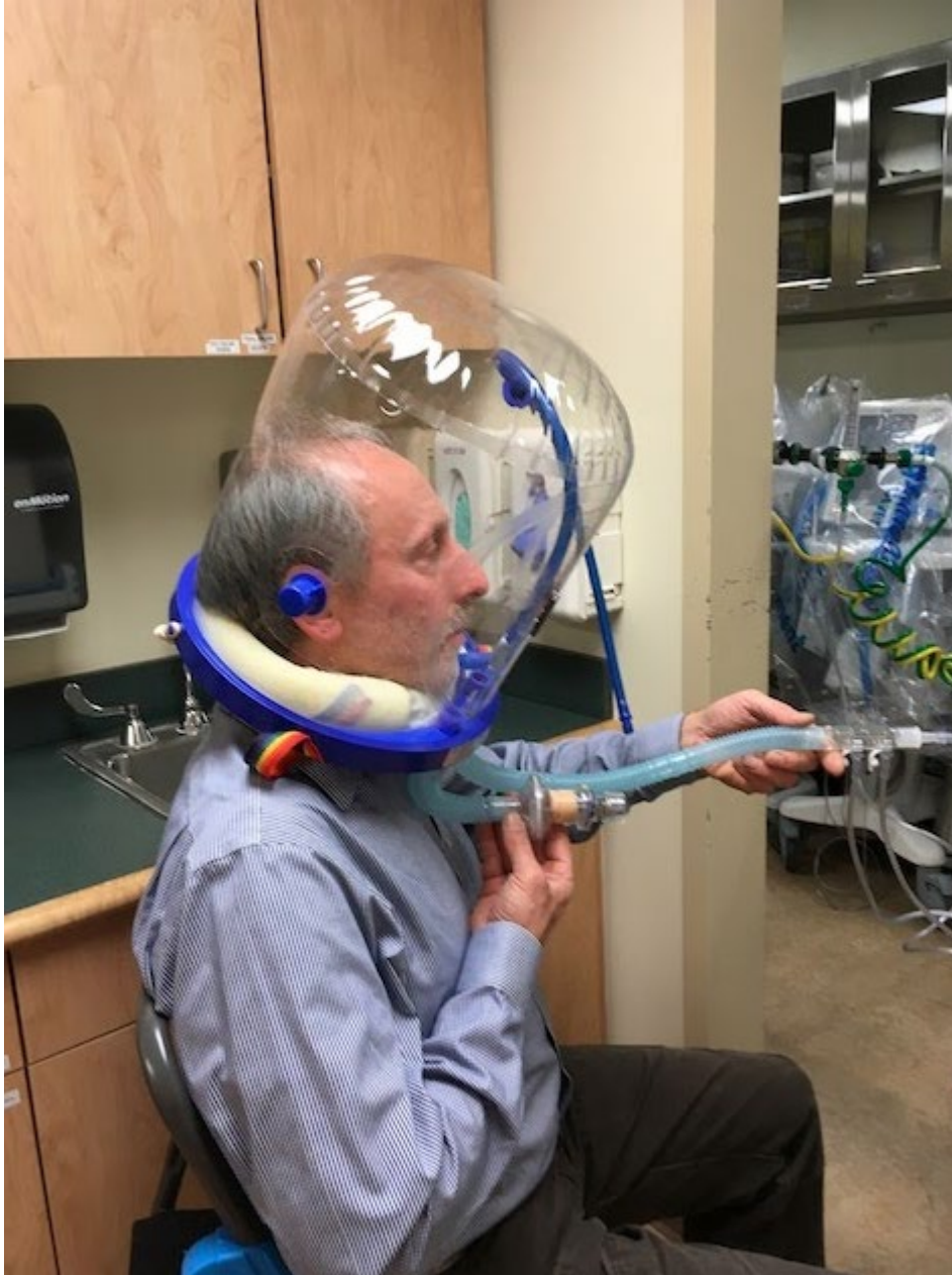
Figure 2: This photograph shows a wall gas driven helmet noninvasive ventilation system, modeled by John Selker, Ph.D. In his right hand (center of photo) is the expiratory circuit with an in-line filter followed by an adjustable PEEP valve. In his left hand (right of photo) are three lines of flush wall gases delivering 100-150 LPM to the inspiratory circuit.
